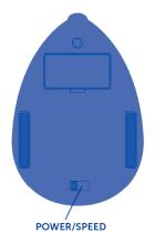
Turn Robot Mouse off by sliding the power button on the bottom.
